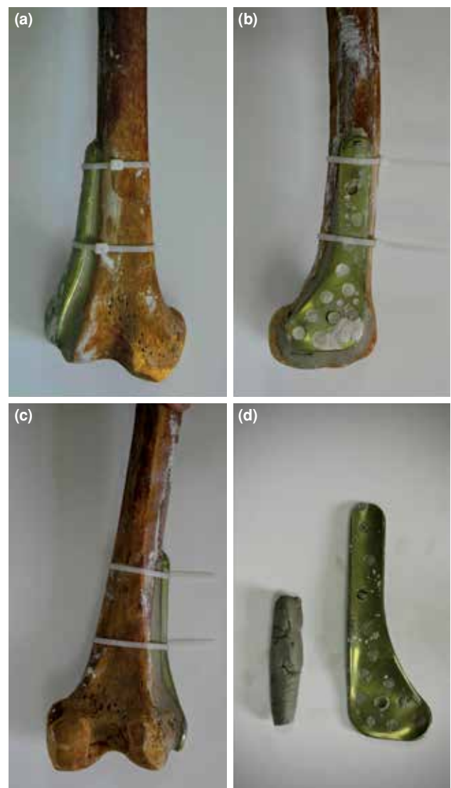
Figure 1. A five-hole Zimmer Biomet Incorporated plate placed in most fitted position as is implemented in actual surgery. (a) Anterior view. (b) Lateral view. (c) Posterior view. (d) Clay between bone and plate was scraped completely and rolled into a ball.
