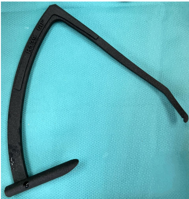
FIGURE 4. Final printed patient-specific guide in polyamide.
