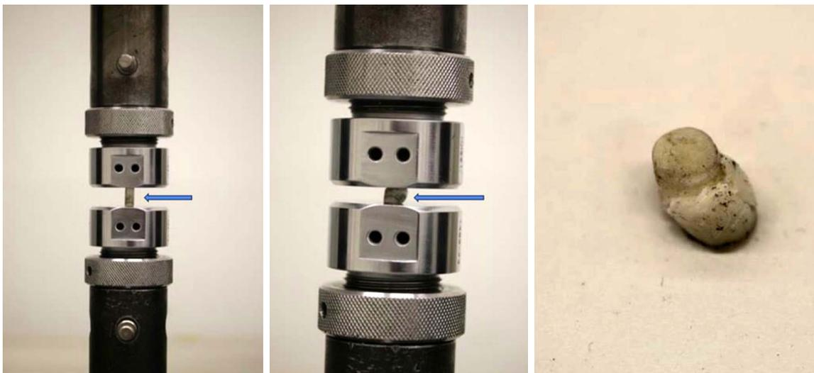
**FIGURE 3.** Compressive load test machine. A cement block (arrow) was secured between the two arms of the machine, which compressed the cement block at a rate of 25 mm/min. The maximum compressive load was automatically measured when the cement block was crushed.
