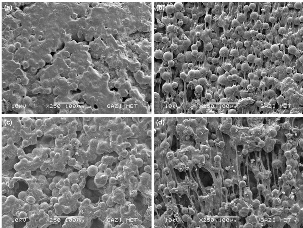
**FIGURE 4.** The electron microscope image shows cement with boron groups at  $\times 250$  magnification, (a) depicting Control, (b) 1 g, (c) 1.5 g, and (d) 2 g.
