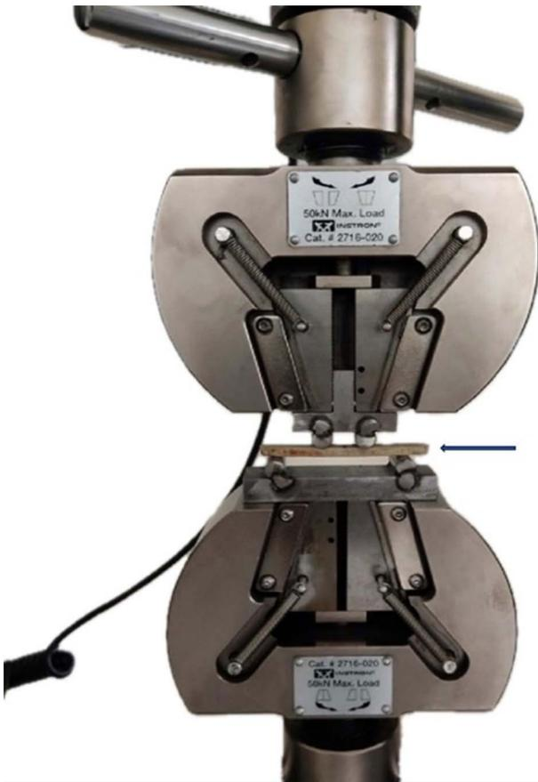
**FIGURE 2.** Four-point bending load test machine. A cement block (arrow) was sandwiched between the for fixtures. The speed of the device was set to 5 mm/min. The maximum four-point bending load was automatically measured when the cement block was fractured.
